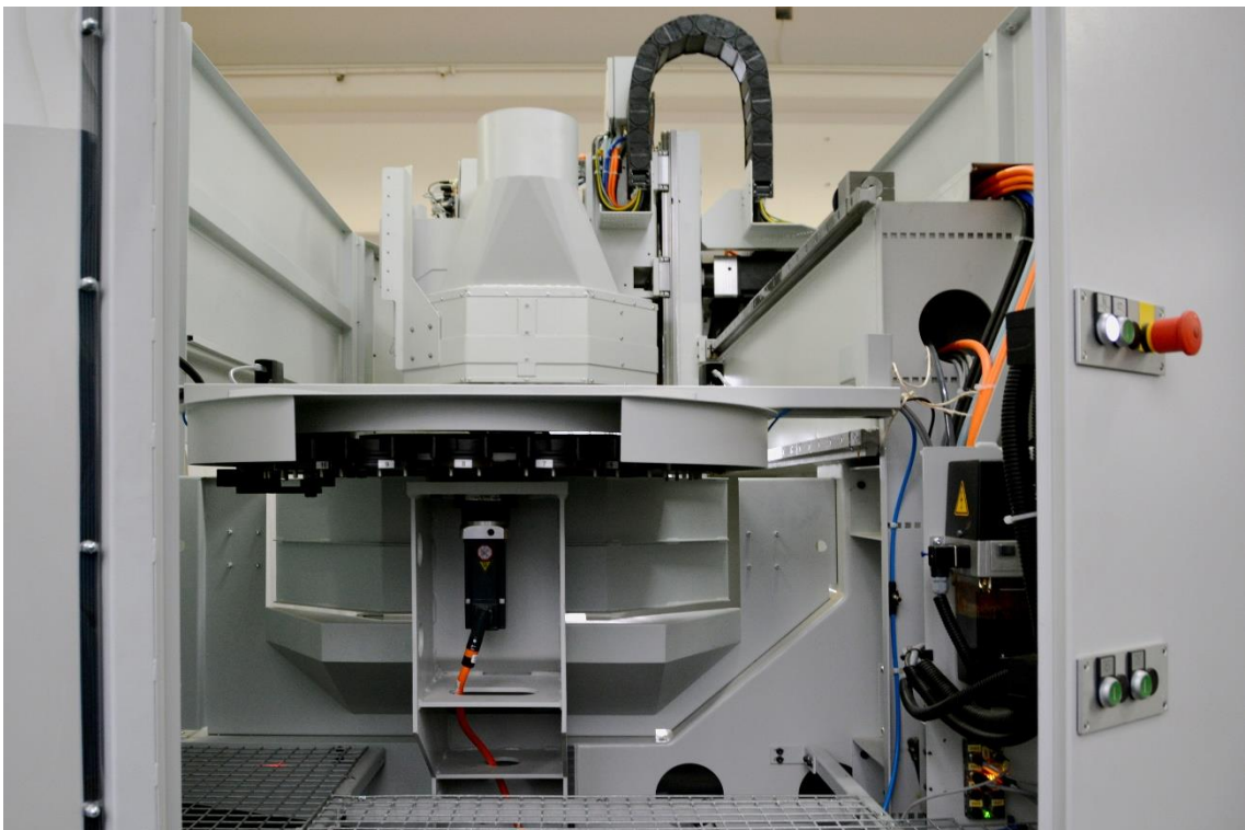
Automatic disk changer for 15 tools attached to the rear of the portal, moves along the longitudinal axis.
