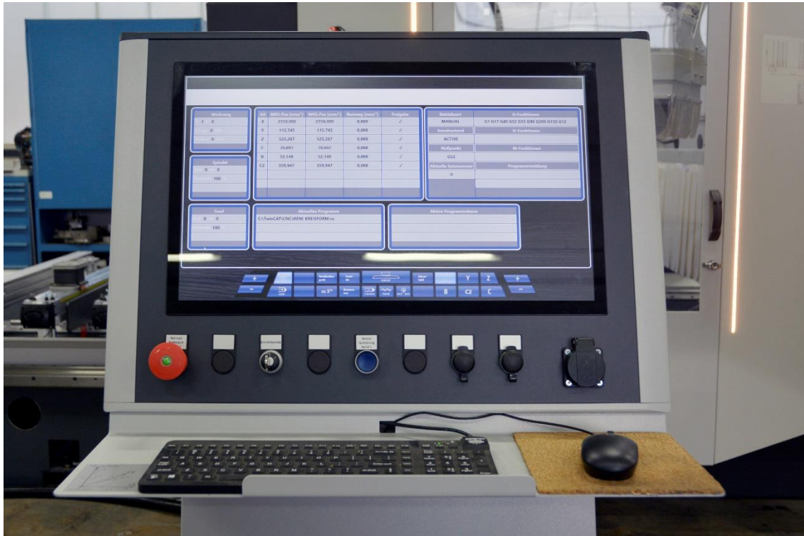
Control: Beckhoff C6015-0010. Reichenbacher WOP user interface.
