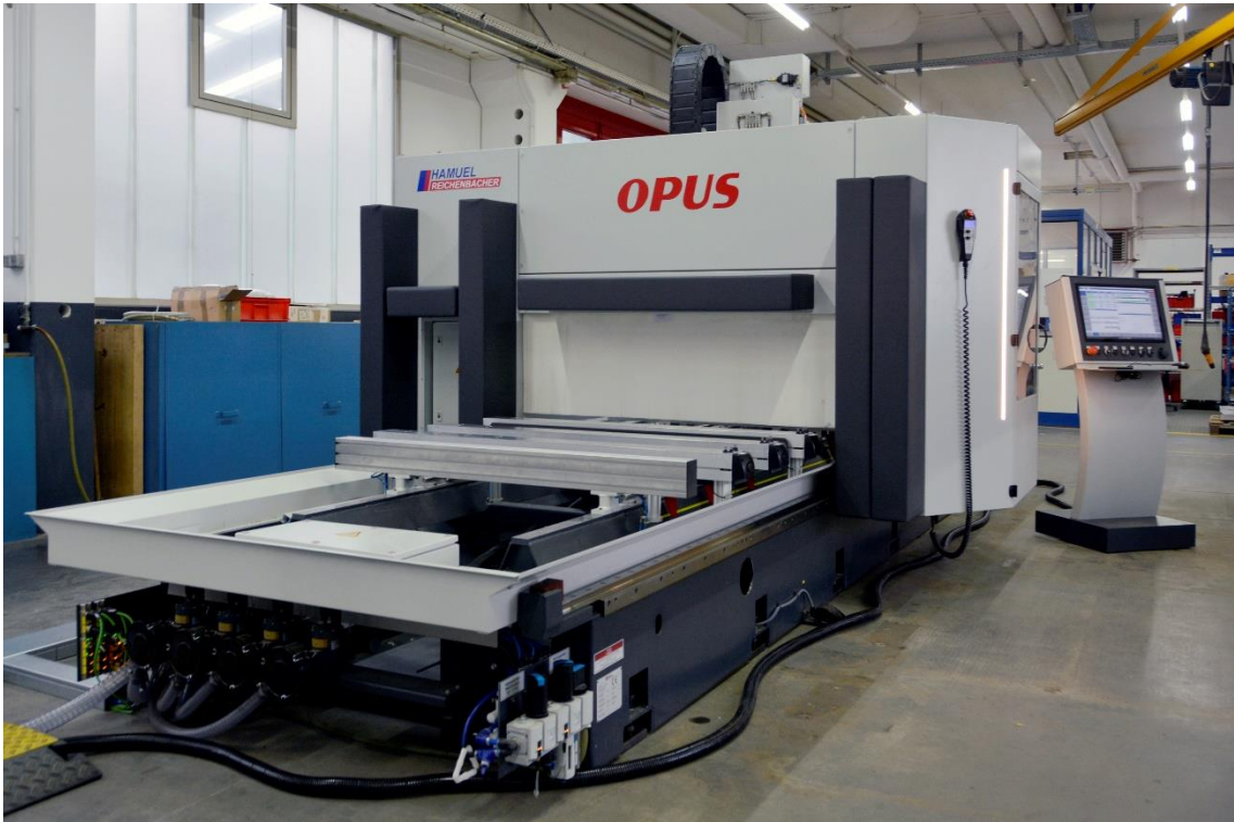
Maximum workpiece dimensions with standard equipment: 5,200 mm x 1,450 mm x 200 mm.
