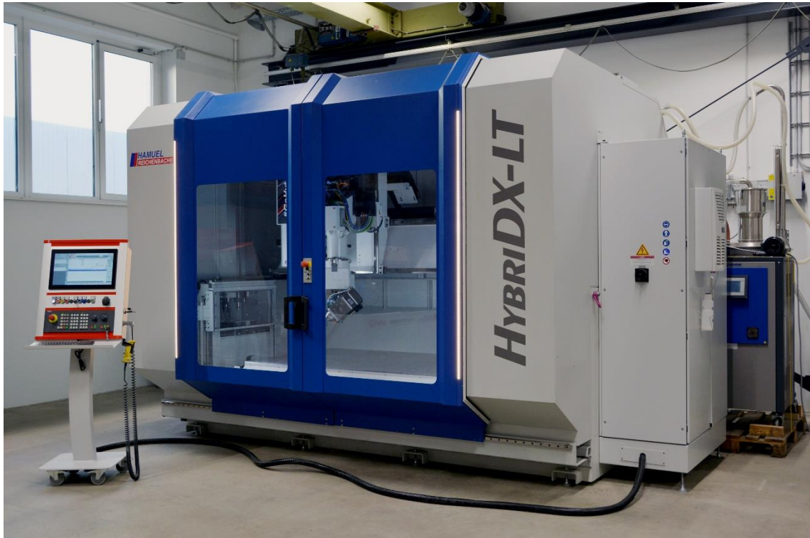
Fixed, low-vibration portal frame construction with integrated fixed machining table.
