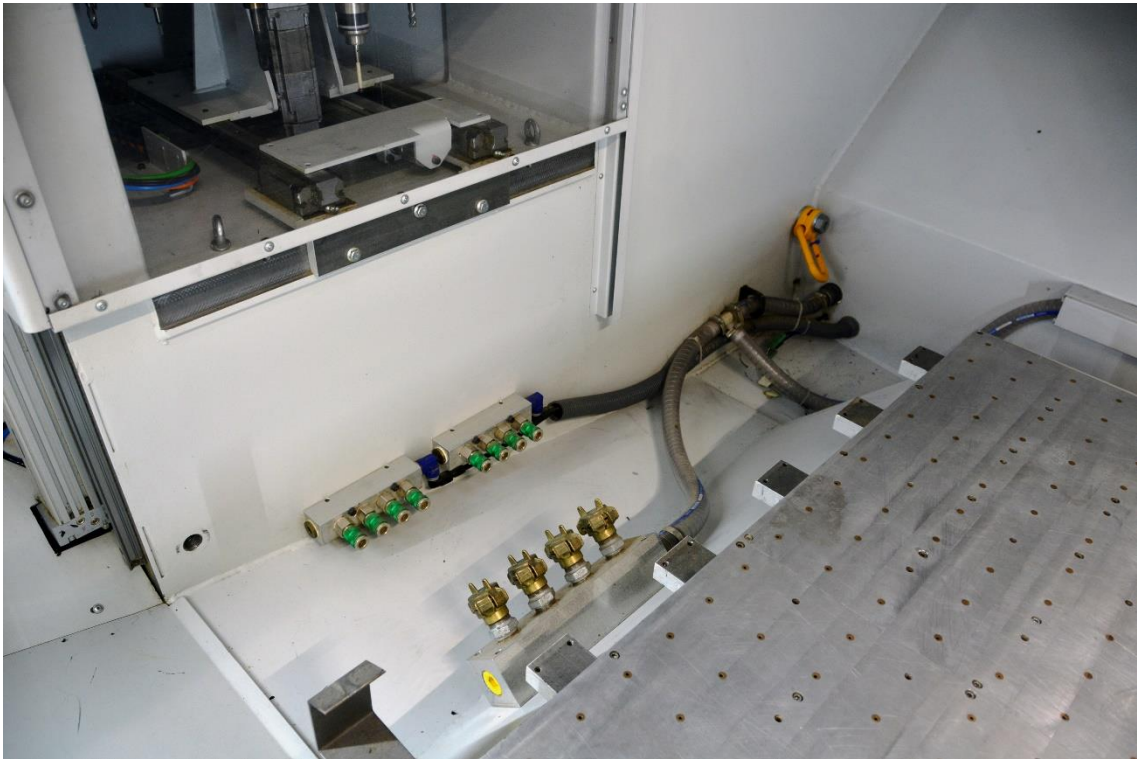
Pneumatic distributor with 4 connections on the left and right in the front table area.
