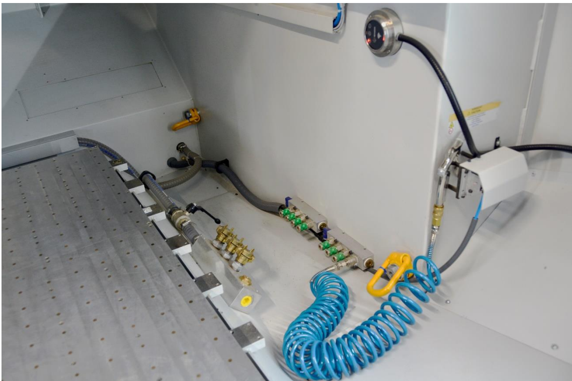
Additional equipment: Simplified tool breakage monitoring on the right-hand side inside the machine.
