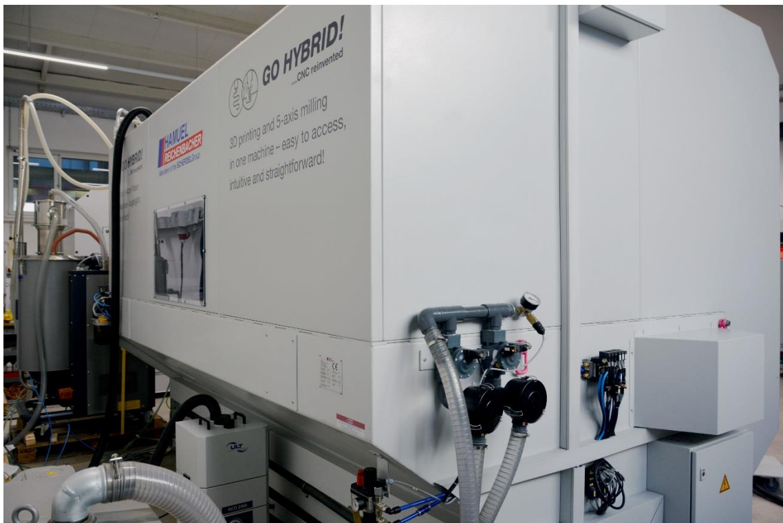
Additional accessories: Cooling unit for milling spindle, air conditioning unit in control cabinet, dry air material dryer.
