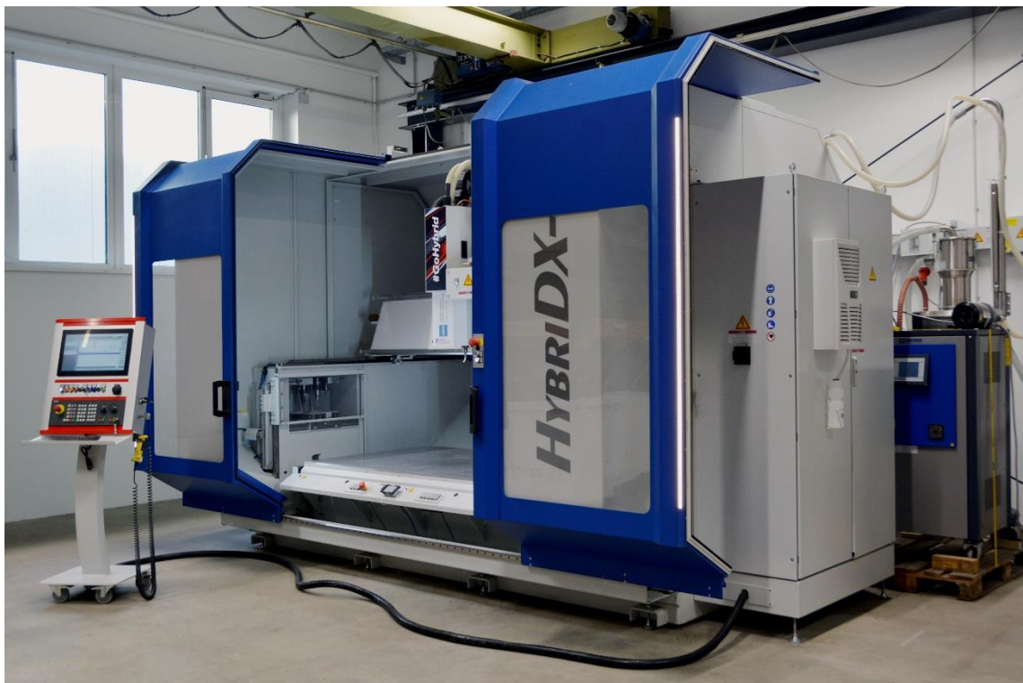
Suitable for additive manufacturing of thermoplastics with and without CF/GF.
