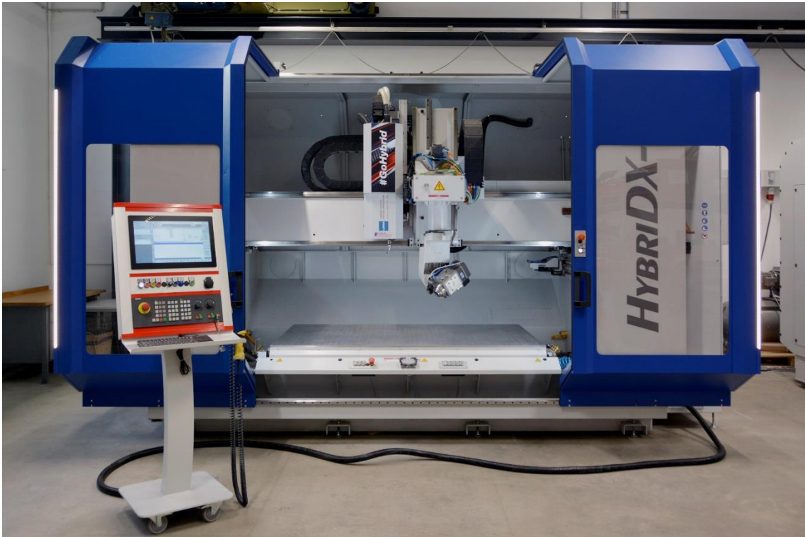
Machining dimensions in X/Y/Z: 1,885 (1,700) x 900 x 600 mm.
