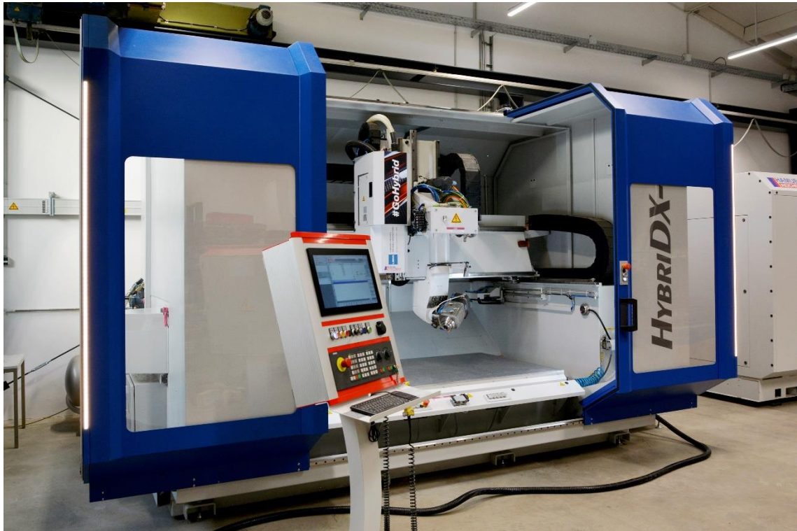
The HybriDX-LT combines industrial 3D printing with precise 5-axis machining.
