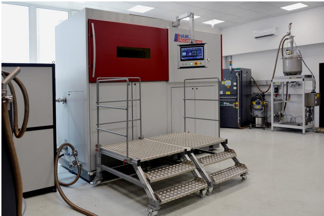
With integrated powder preparation and protective gas system.
