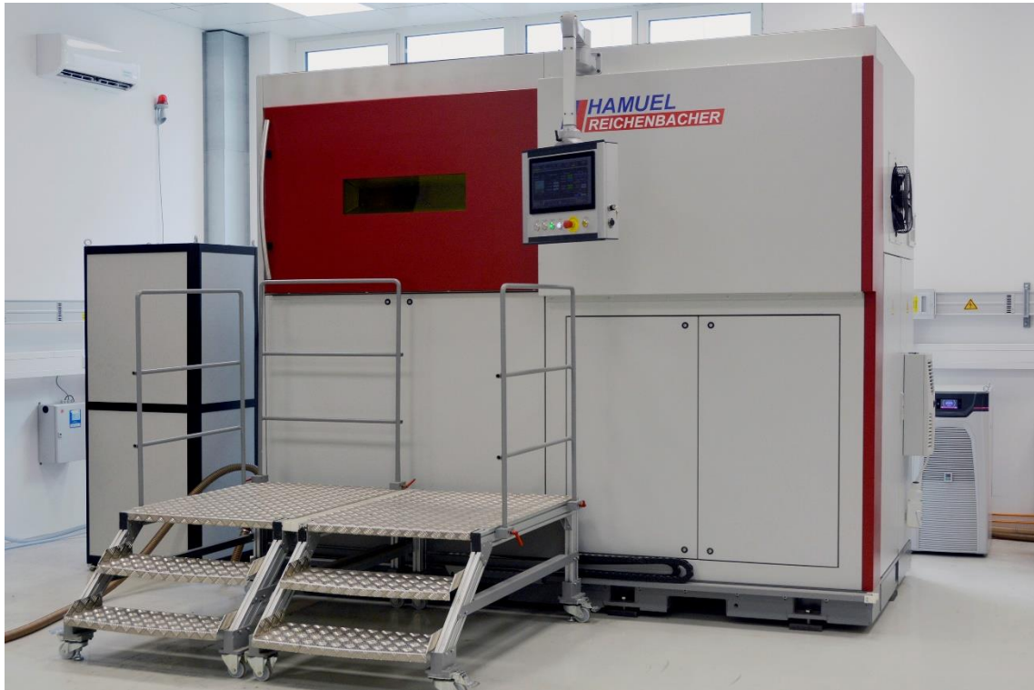
Components are manufactured on the AMS 400 using the L-PBF process (selective laser melting).
