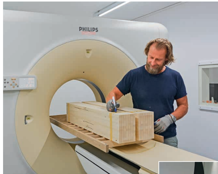
The spruce wood is inspected using computerised tomography.
