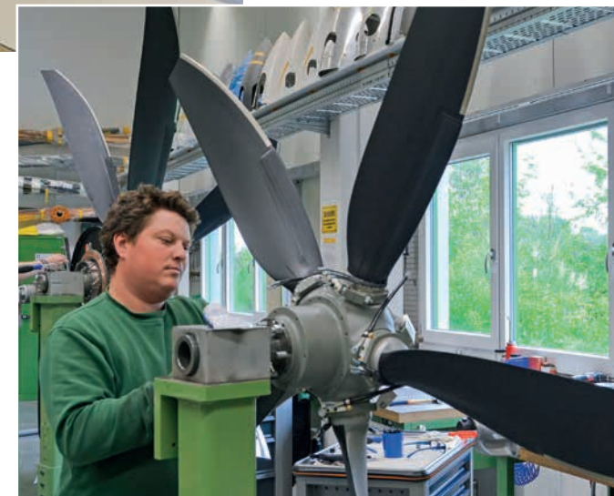
Different profile thicknesses, variable blade angles and complex twists create highly dynamic three-dimensional free-form surfaces.
