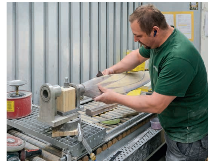
Around 70 per cent of the grinding processes, which require precision to within a tenth of a millimetre, are still carried out manually.
