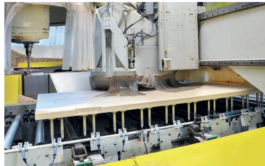
CNC system type VISION-II-UT with portal loading system.
